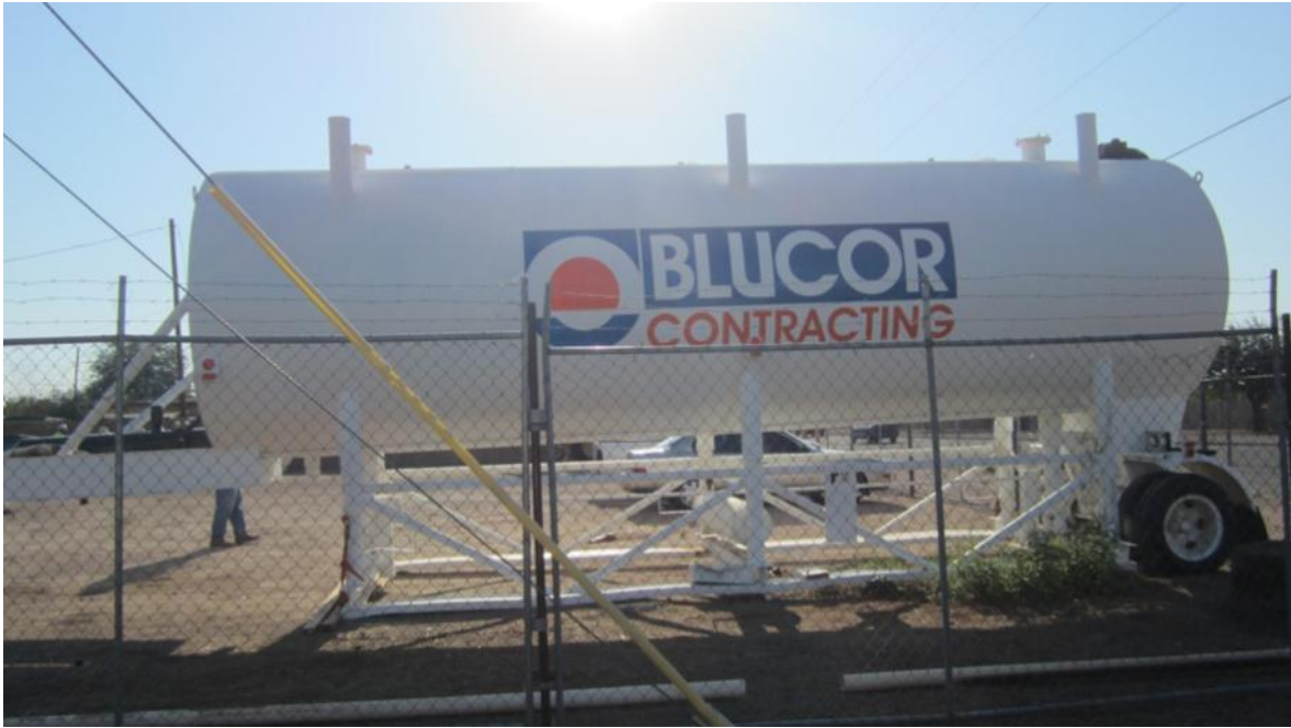
Water trailer for dust control
